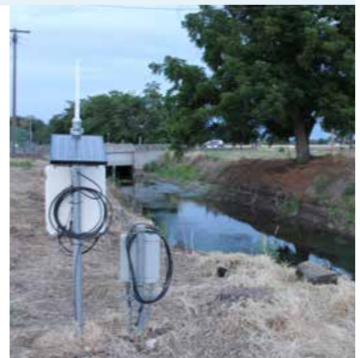
A solar-powered stream gauge measures water levels near Gardena, Washington
